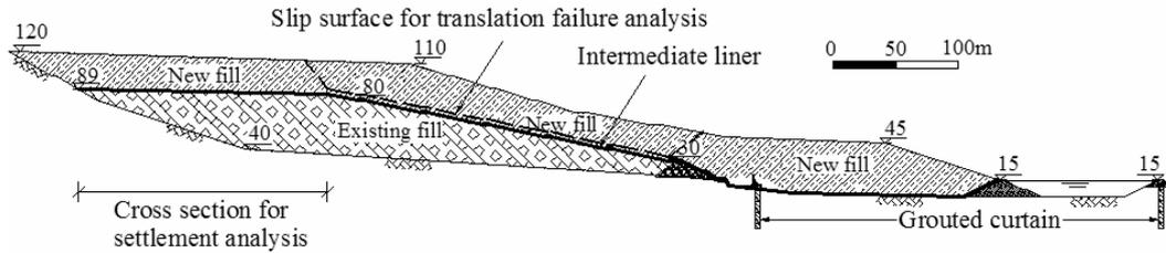
Figure 1. A preliminary design of landfill expansion in Suzhou, China
