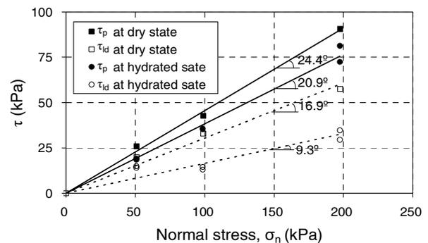
Figure 6. shear strength envelopes for the GCL/GM interfaces
