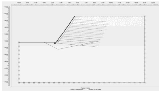
Figure 5. Plastic zone at the slope toe, after the lowermost nail is installed.
