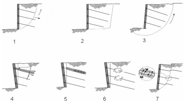
Figure 1. Ultimate limit states (ULSs) of reinforced soil massifs (Lazarte et al, 2003).
