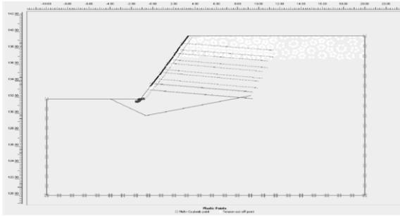
Figure 4. Plastic zone at the slope toe, before the lowermost nail is installed.
