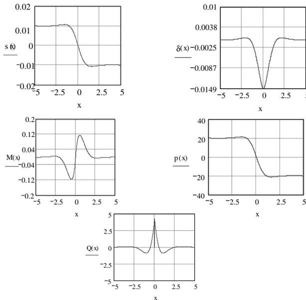
Figure.2. Displacements  $s(x)$ , inclinations  $\delta(x)$ , bending moments  $M(x)$ , shear forces  $Q(x)$ , soil reactions  $p(x)$  (tons and meters)
