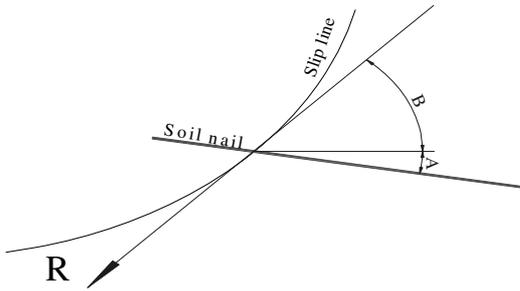
Figure 3. Soil nail, crossed by slip-line
