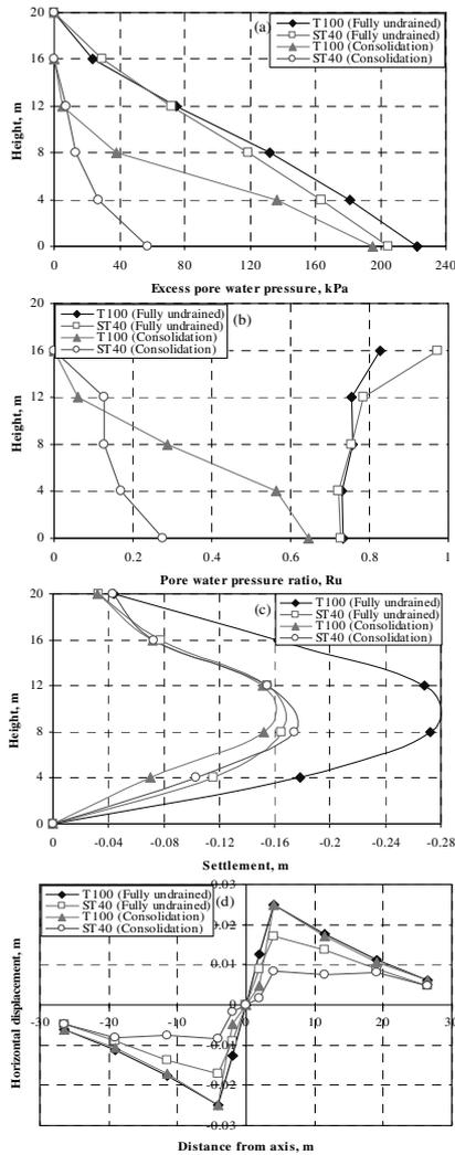
Figure 5. Variations of: (a) excess pore water pressure, (b) pore water pressure ratio, (c) settlement, and (d) horizontal displacement along the core height
