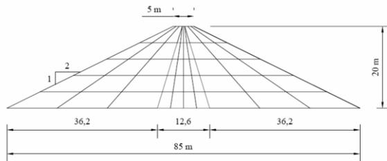
Figure 3. Geometrical characteristics and finite element mesh of the dam.
