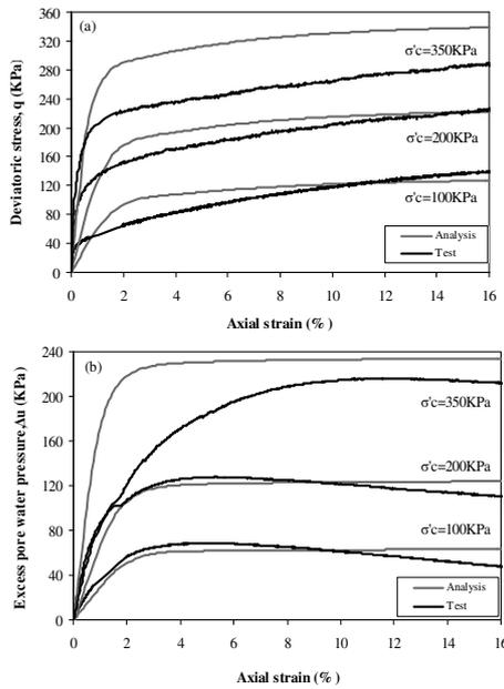
Figure 2. Tests and analyses results of ST40 specimen: (a) deviatoric stress, and (b) excess pore water pressure.
