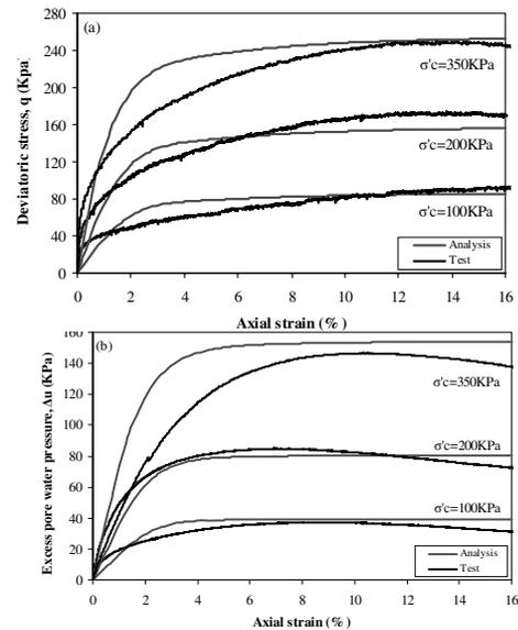
Figure 1. Tests and analyses results of T100 specimen: (a) deviatoric stress, and (b) excess pore water pressure.
