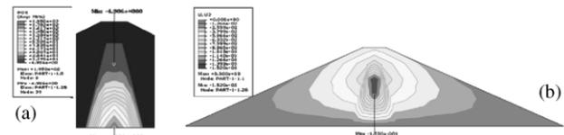
Figure 4. Contours of construction-induced (a) excess pore water pressure and (b) settlement of the earth dam with pure clay core, when core consolidation is allowed.
