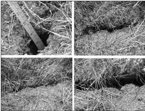
Figure 6. Desiccation cracks along construction joint.
