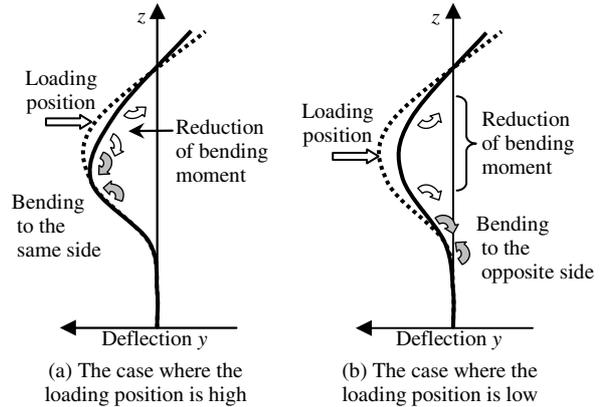
Figure 6. Difference in the change of deflection of sheet pile caused by the loading position
