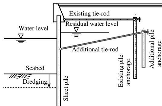
Figure 1. Example of dual-anchored sheet pile wall
