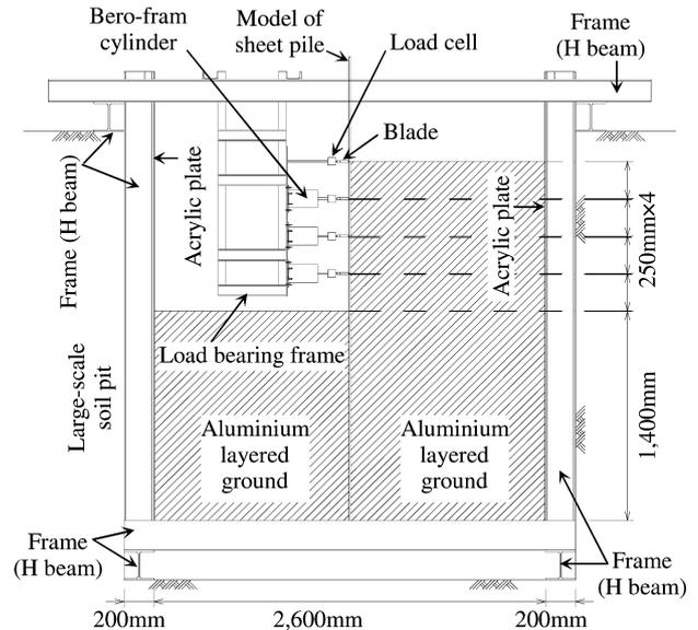
Figure 2. Model of dual-anchored sheet pile wall
