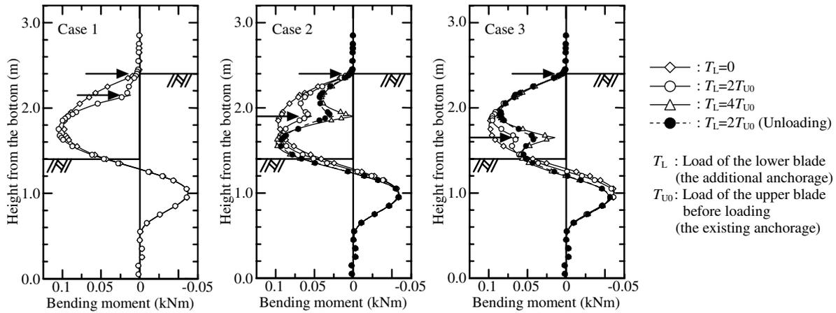
Figure 4. Changes in distributions of the bending moment induced by loading of the additional anchorage
