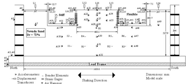
Figure 1. Section through the model showing the position of the model structures and the layout of instrumentation. Dimensions in model scale (mm).
