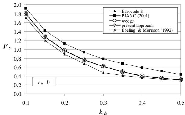
Figure 5. Effect of  $k_h$  on sliding stability.
