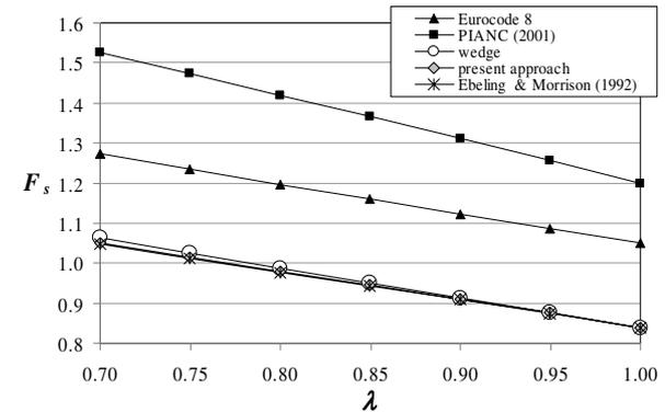
Figure 3. Effect of level of submergence on sliding stability.
