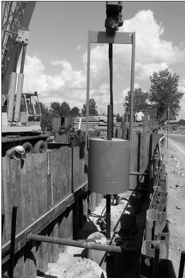
Figure 2. Dynamic load test of bored pile \phi 1500 mm using vibrating hammer and hammer weight 92 kN.
