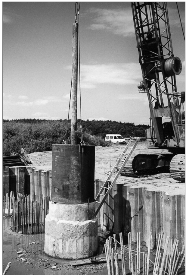
Figure 1. Dynamic load test of bored pile \phi 1500 mm using hammer weight 50 kN and the crane with free release of the rope.
