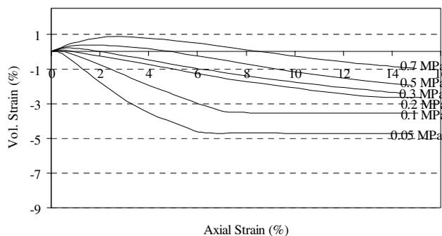
Figure 2. Variation of volumetric strain versus axial strain for different confining pressures
