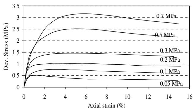
Figure 1. Variation of deviatoric stress versus axial strain for different confining pressures
