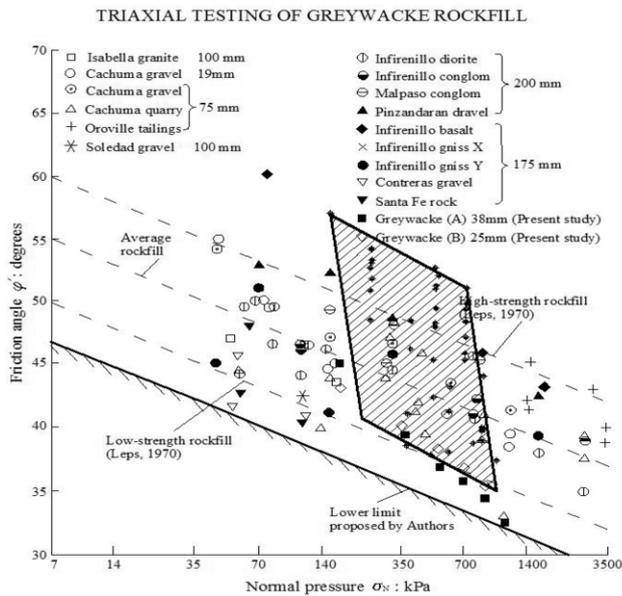
Figure 4. Friction angle versus normal pressure (Indraratna et al 1993)
