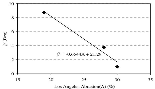
Figure 7. Dilatancy angle versus abrasion weight loss at  $\sigma_3=300kPa$
