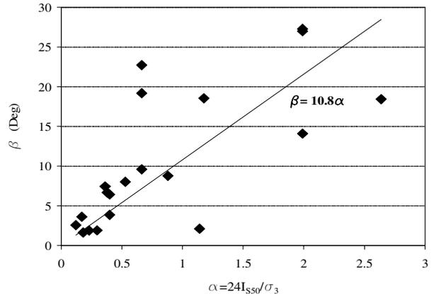
Figure 6. Dilatancy angle versus  $I_{S50}$
