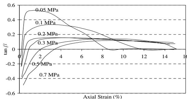
Figure 3. Dilatancy angle versus axial strain for different confining pressures
