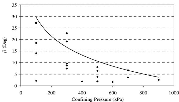
Figure 5. Variation of dilatancy angle versus confining pressure
