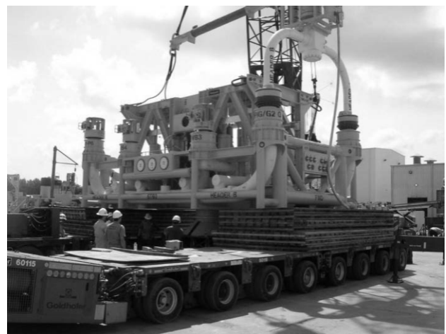
Figure 1. Manifold for a field development in the Gulf of Mexico. (Photo: Stephen Reid, Aker Solutions)
