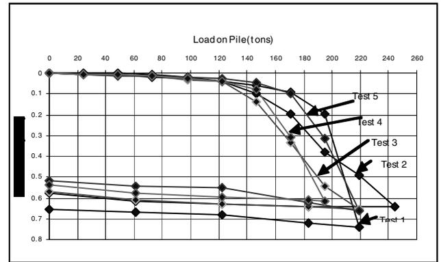
Figure 1 Load settlement plots for five pile load tests
