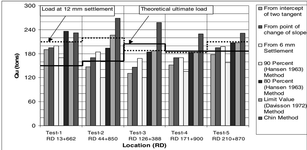
Figure 2 Variation of ultimate load for each pile using different methods
