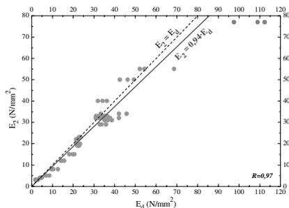
Figure 3. Correlation between B&C and static plate load test moduli
