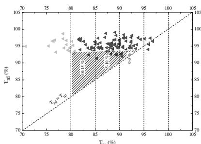
Figure 4. Compaction values measured by B&C ( $T_{rd}$ ) and by conventional method ( $T_{rp}$ )
