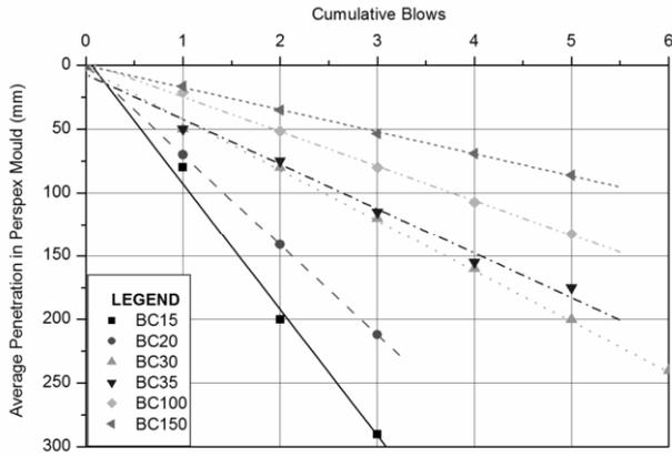
Fig. 6. Cumulative blows penetration tests for DCP Test
