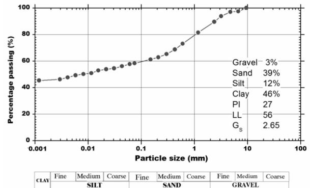
Fig. 2. Grading characteristics for test material
