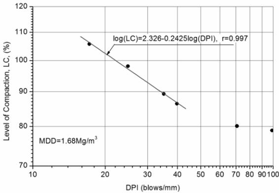
Fig. 7. Relationship between Level of Compaction and DPI
