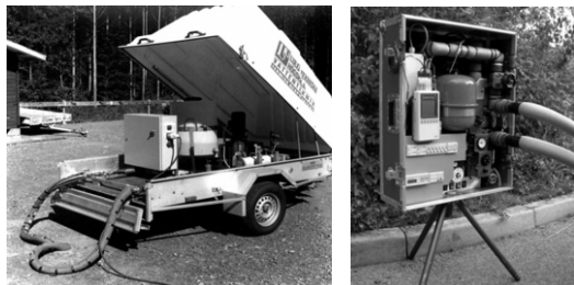
Figure 3. Left: first GRT equipment, Lulea University of Technology, Sweden (Gehlin 2002) Right: enhanced mini GRT module, École Polytechnique Fédérale de Lausanne, Switzerland (Laloui & Steinmann 2005).
