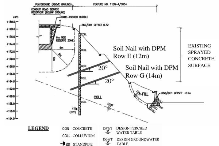
Figure 1. Geological model of Feature No. 11SW-A/CR34.
