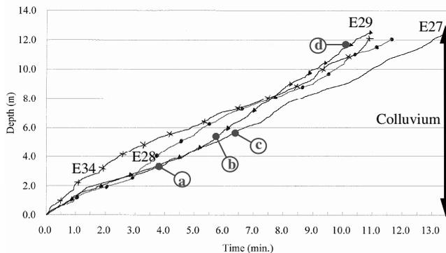
Figure 3. Depth vs Time Graph of DPM Results for Feature No. 11SW-A/CR34 (Soil Nail Row E).
