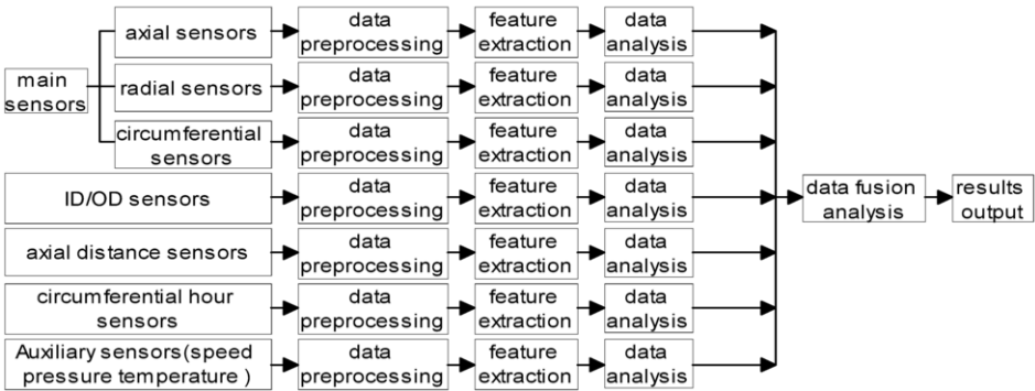
Figure 6. Fusion analysis structure of magnetic flux leakage detection data
