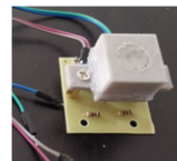
Fig.7. The probe for the lay length detection
