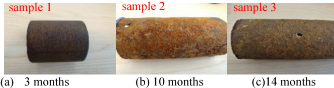
Figure 1. Corrosion samples of Q235 steel with different service periods
