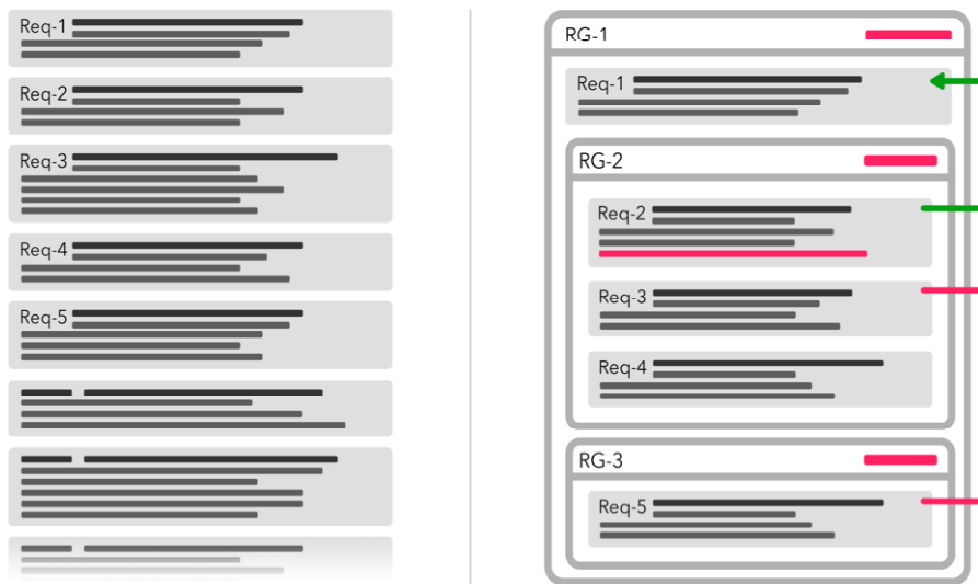
Figure 1. Schematic view of the representation of the requirements at the starting point and in the as-is situation in scene. The left side shows a list of requirements without hierarchical order and variance information. The right part of the figure shows the requirements aggregated in requirement groups with colored variance (excludes and implies) information.
