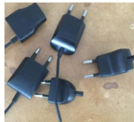
Figure 3. Hand-made prototypes of power supply cover.
