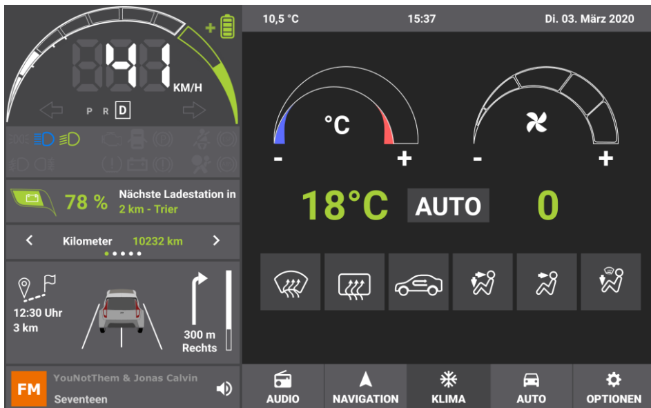
Figure 1. Display-based UI of the human-vehicle interface Android prototype “evoDash” with the climate control screen currently displayed on the right and dynamic driving data displayed on the left.
