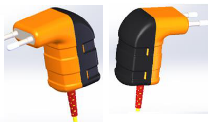
Figure 28. Version II of vertical parting plane of the form.
