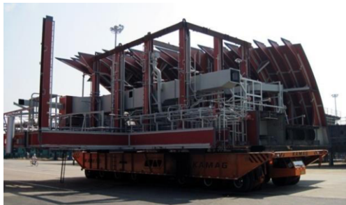
Figure 1. Transport ship block by a flatcar.
