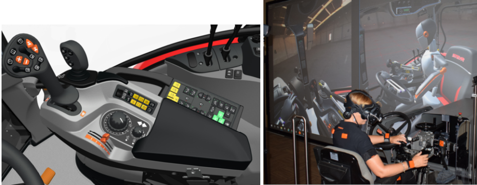
Figure 4. New armrest layout based on intuitive-grouped control panels (left) and immersive tests in Virtual Lab (right).
